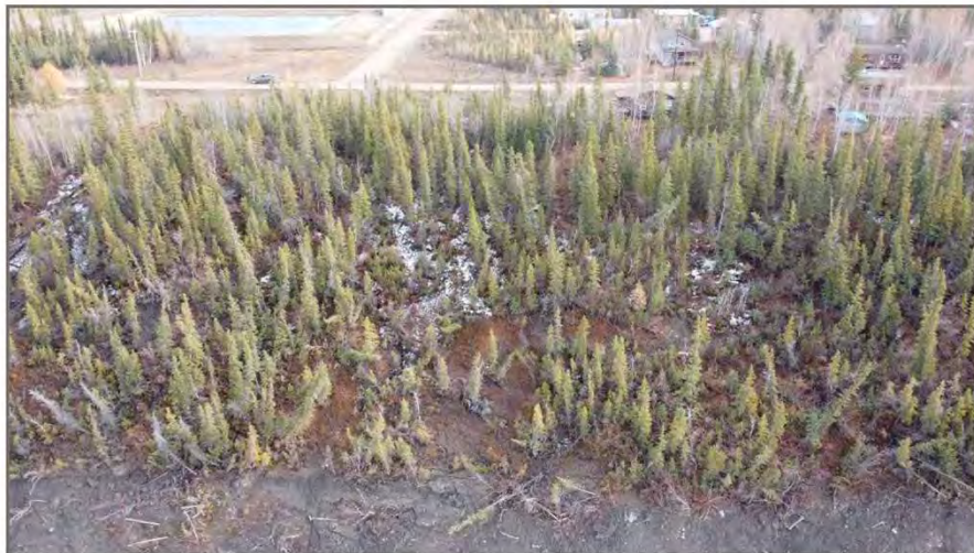
Photo 42: House 1S: aerial view, top of photo is east. Large, approximately 60 m long, backscarp halfway down the upper vegetated portion of the riverbank slope.
